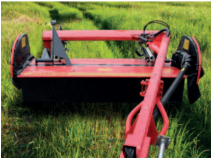
The side guards are easily folded upwards.
