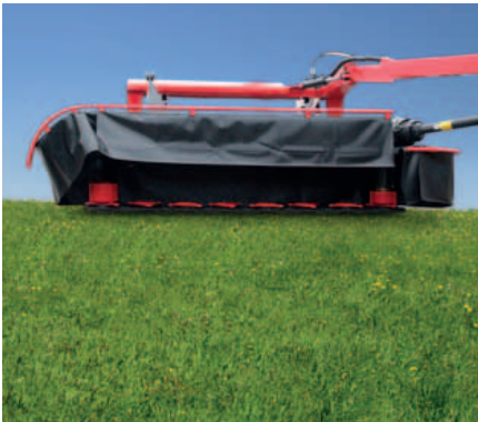
Easy access to the cutterbar for service and maintenance.
