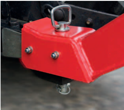
EXTRA 532 and EXTRA 540 are easy to connect to a tractor with a simple pin system.
