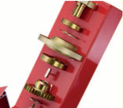
To protect the gear wheels and the drive system, a one-key safety device is used, designed to break in case of overload.
