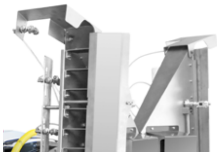
Structure to divert the flux of air for treatments near houses
